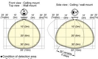
Condition of detection area Detection timer: 0.2sec. Origin of flame: Gas lighter
